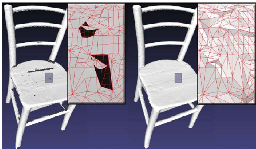
Figure 2.6: The raw model of a chair with defects (left). The same model repaired with the Attene’s algorithm (right) (Figure taken from [7]).
